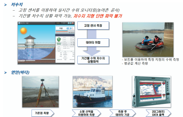
Fig. 4. Conventional survey method of reservoir/coastal(ocean).
