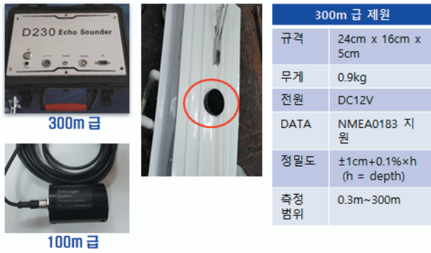
Fig. 7. Single beam echo sounder specifications.
