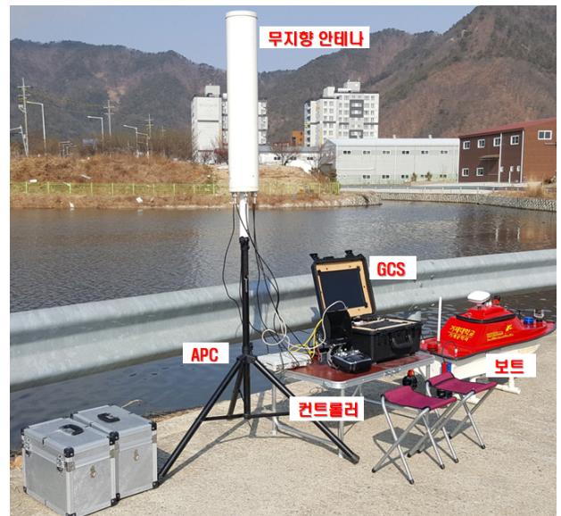
Fig. 3. USV for explore the ocean floor and geographical surveying.
