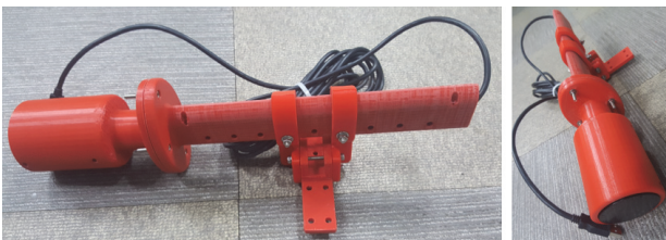
Fig. 5. Single beam echo sounder mounted on jig printed 3D printer
