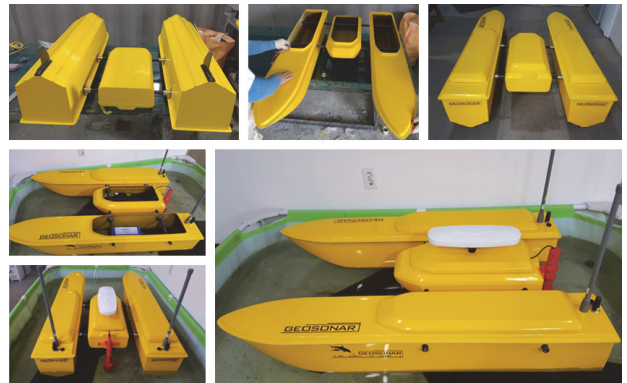
(a) Hull production and balance test
