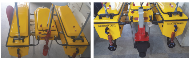
Fig. 12. Jig structure for mounting SONAR
