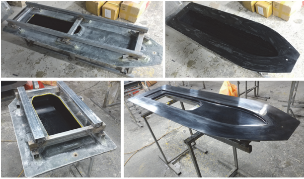
Fig. 8. Mold for hull production
