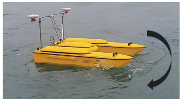
Fig. 11. Turning test in sea area (clockwise rotation)
