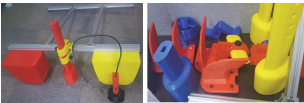
Fig. 4. Design verification using 3D printer
