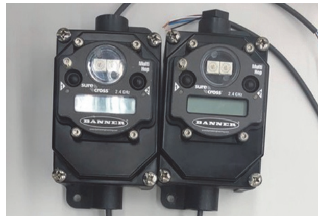
Fig. 9. Gateway and node of the vibration monitoring and data saving system
