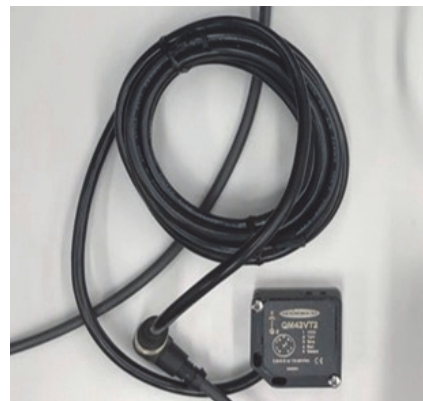
Fig. 8. Sensor of the vibration monitoring and data saving system
