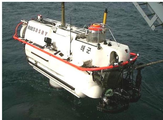
**Fig. 1.** Deep Submergence Rescue Vehicle (DSRV)
