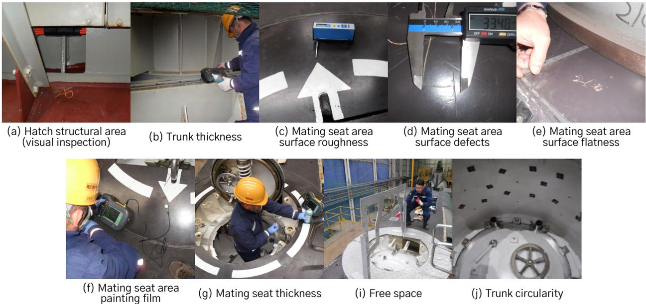
Fig. 4. Submarine Rescue Hatch Area Inspection & Certification (SRIC) procedure
