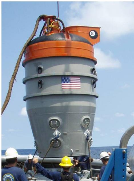
**Fig. 3.** Submarine Rescue Chamber (SRC)
