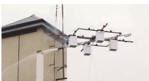
(c) Drone for firefighting
