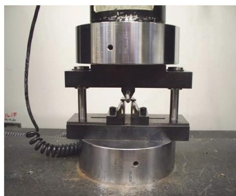
Fig. 5. Short beam shear test fixture and Instron 5583
