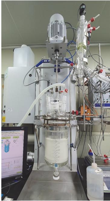
Fig. 2. Reaction Calorimeter(RC-1e)
