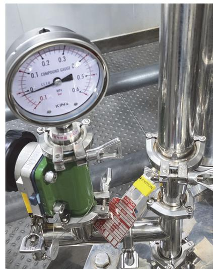
Fig. 11. Rupture disc system on top the synthesis reactor
