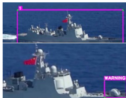
Fig. 6. Identification, classification for weapon system and activation of display warning message
