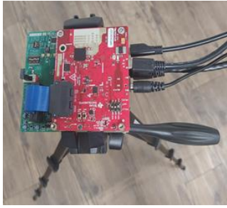
Fig. 6. TI IWR1843 FMCW RADAR
