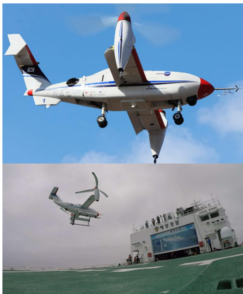
Fig. 2. High-speed VTOL(vertical take-off and landing) UAV(top) and maritime takeoff and landing of a tiltrotor UAV(bottom)[9]
