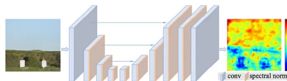
Fig. 5. Architecture of the U-Net discriminator with spectral normalization[13]
