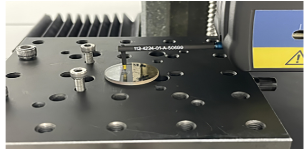
Fig. 15. Measurement of Au coating thickness
