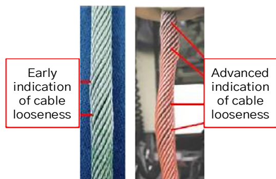
Fig. 6. Examples of wire rope cable looseness[10]
