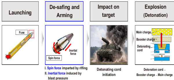
Fig. 4. Principles of ammunition fuzes[3]
