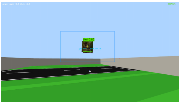
Fig. 6. YOLO-based bird detection with digital zoom crop
