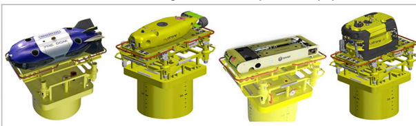
(c) Subsea docking station
