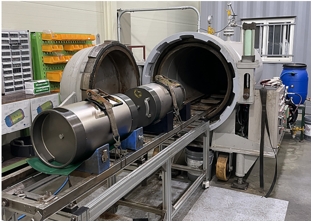
Fig. 6. Hydrostatic pressure test
